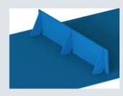
Gussets can be welded to the reverse of the cleat to provide support. Gussets should be positioned according to the width of the cleat, the load supported and its distribution on the cleat.
